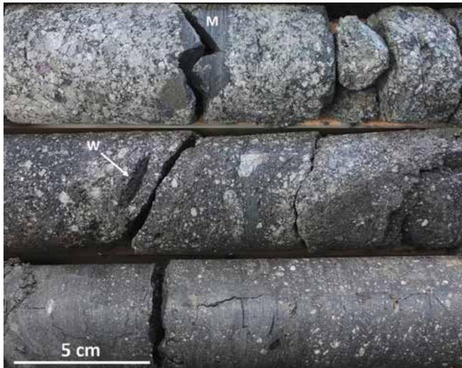
Figure 3: Photographs of drill core from the Bear kimberlite illustrating the variation in olivine concentration and grain size. The pale grains are variably altered olivine and occur within a dark very fine-grained matrix dominated by mud. A plastically deformed clast of mudstone (M) and a fragment of carbonized wood (W) are also evident.
